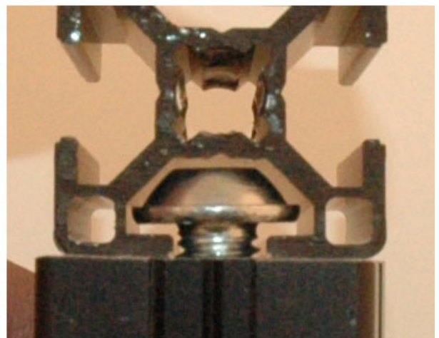
Safety screw not touching top (correct)
